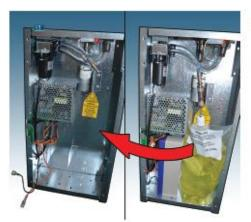
Insert the plastic bag in the compartment as shown in the picture
